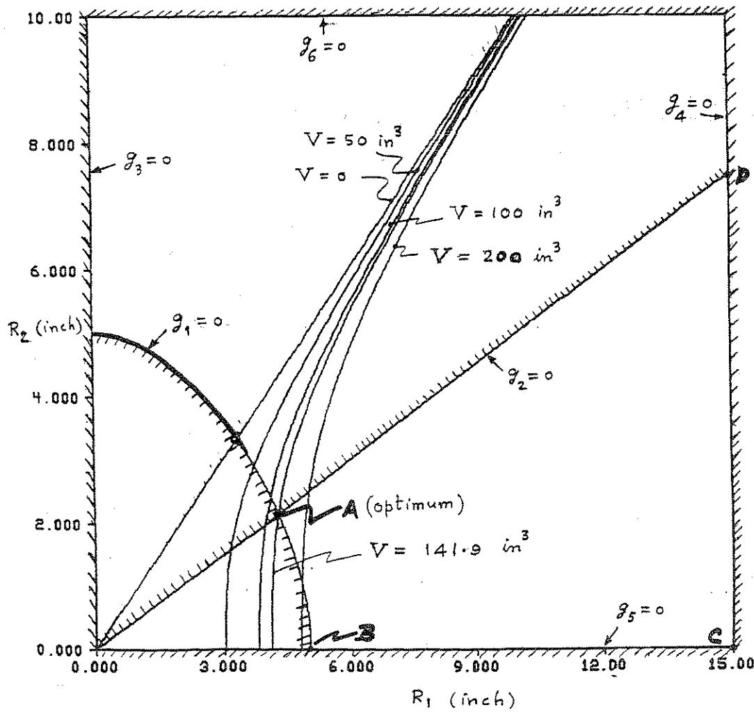
(b) Constraints = same as in part (a) except that  $g_2$  is changed to  $R_1 - 2R_2 \leq 0$ .
